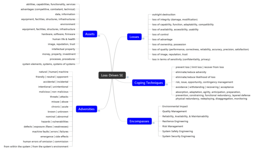
Figure 1: Attributes and Scope of the Integrated Loss-Driven Systems Engineering Problem Space
